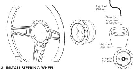
Position steering wheel on adapter and install nine 8-32 flathead screws, tighten down steering wheel. Check the steering wheel to make sure it is straight. To adjust, remove the assembly (steering wheel & adapter) and index the adapter on the splined shaft. Once straight, torque steering shaft nut to 20-25ft. lbs.
