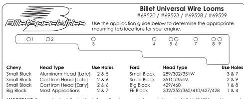
**IMPORTANT:** For center bolt [Late Model] applications, our late model bracket kit (#69600) must be used. **#69528 [Flame]:** Flames will point towards the front of the engine on Ford applications.
