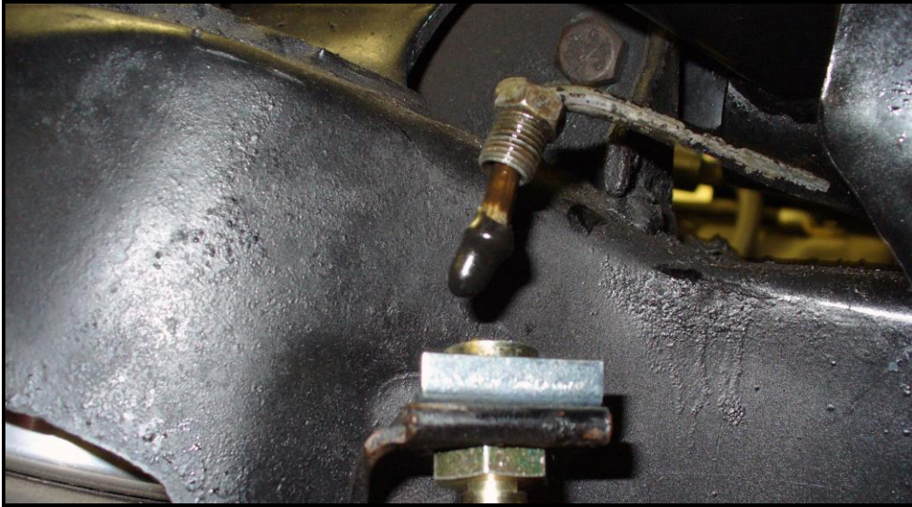
Hose lock location and vinyl cap installed
