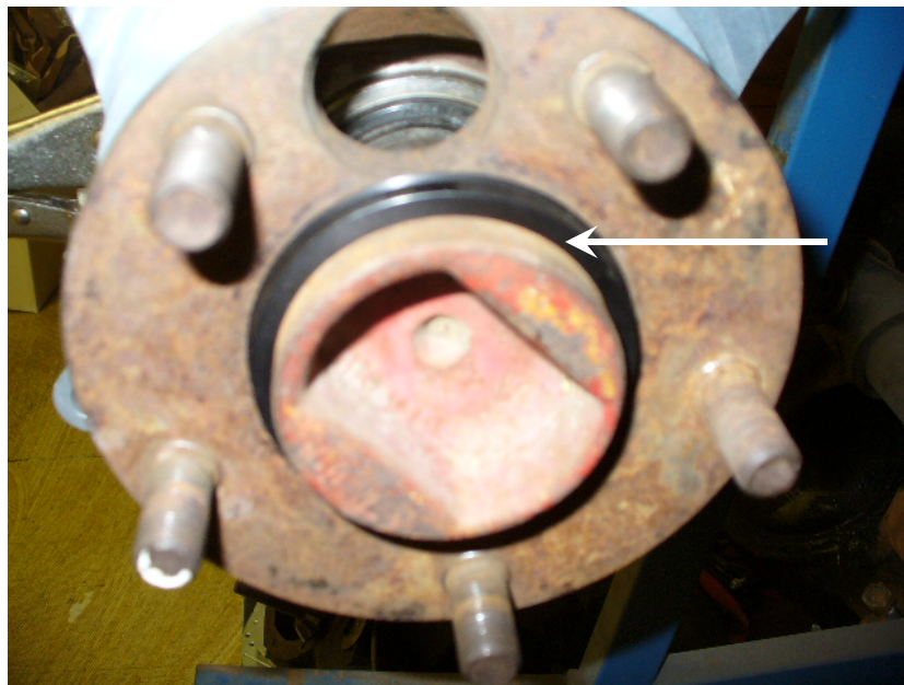
Black centering ring installed over rotor register.
