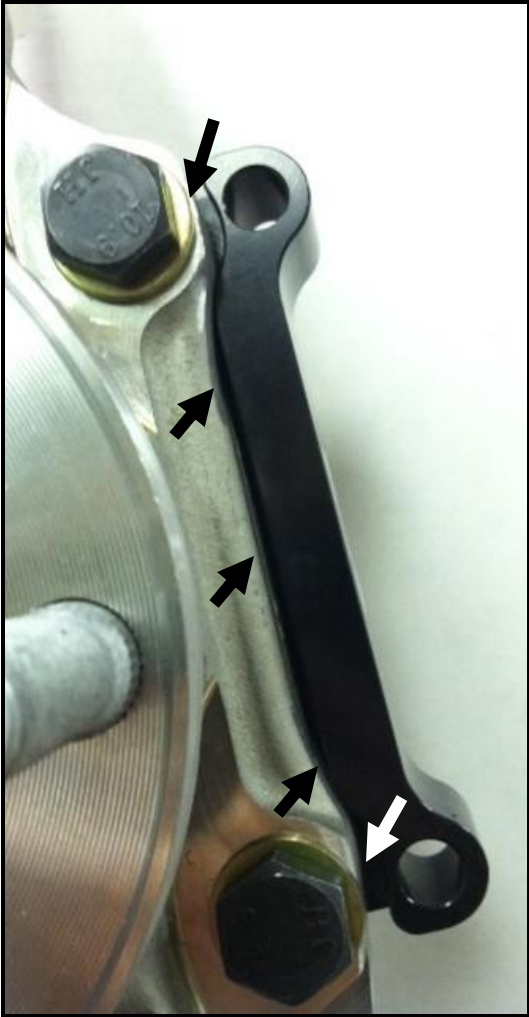
Figure 5: Caliper ears and bracket must clear the indicated areas
