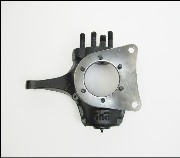
5. Slide the Base bracket over the studs and on to the knuckle.
