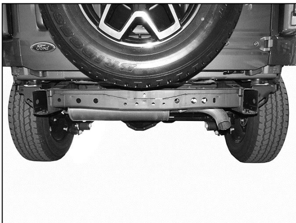
(Fig 3) Remove bumper assembly
