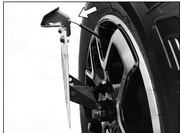
(Fig 22) Plug Harness into license plate light
