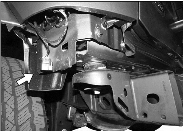
(Fig 1) Unplug all wiring harnesses leading to the rear bumper, (arrow-driver/left side pictured after bumper removal)
