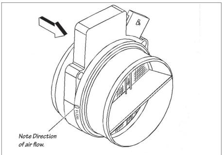
**11.** Install the Banks Filter onto the Banks Ram-Air Filter Cover. Press fit the two pieces together until an audible snap is heard. This process will ensure that a correct seal has been established. Tighten Banks Filter hose clamp.
