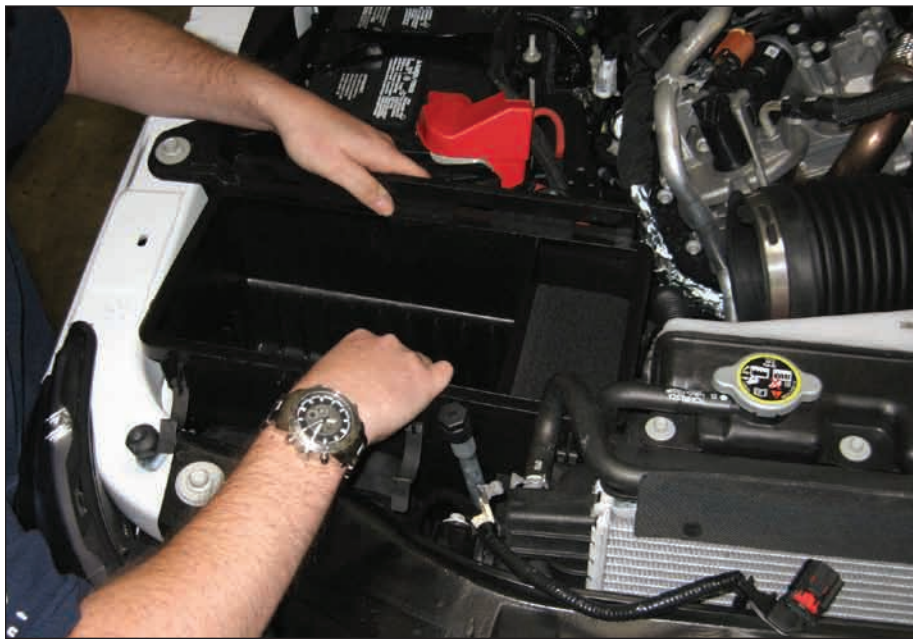
Figure 7- Removal of the stock air filter housing
