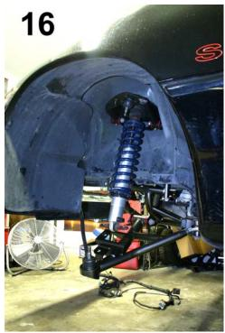
**NOTE**: A rotary file was used to elongate the holes in the lower mount of the strut to properly align with the lower a-arm. This applies to stock lower arms as well. This is common if equipping with **Strange Engineering** coil overs.
