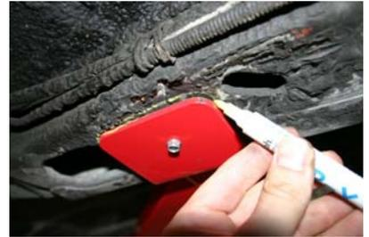
BMR Subframe connectors ship with additional reinforcement plates that may be welded in if desired. They are designed to join the factory pinch welds on the rocker panels to the Subframe Connectors. The reinforcement plates are not necessary for light duty street applications but are recommended for aggressive road racing, high horsepower drag racing applications or when using the BMR Trak Pak or Xtreme Duty torque arms with weld-in cross-member. See image below for installation example.
