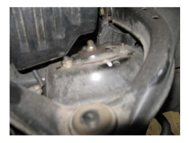
2c. As you did for the top mounts, remove the bottom mounting bolt of the spring/strut assembly.
