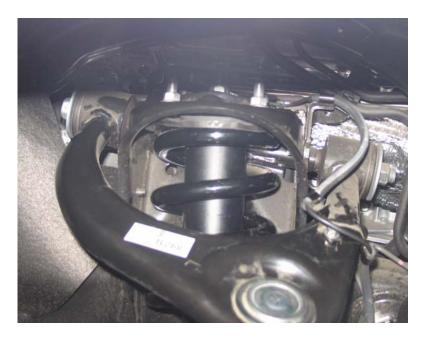
2c. As you did for the top mounts, remove the bottom mounting bolt of the spring/strut assembly.
