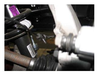
3b. To be able to install the Belltech Lift Strut the lower control arm bolts to the frame must be removed, and the lower control armed lowered from those positions.
