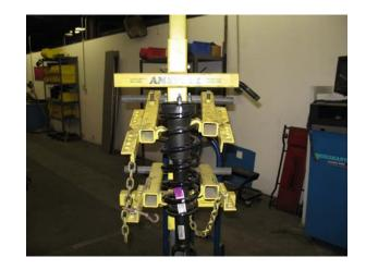
**4b** Before disassembling the strut mark the position of the top mount in relationship to the lower bolthole. Using a spring compressor, compress the spring to remove the pre-load of the spring from the strut. Using the correct tools remove the top mount from the strut. We do not recommend using power tools. Now disassemble the strut and release the spring tension, be sure to remember the order the components are removed.
