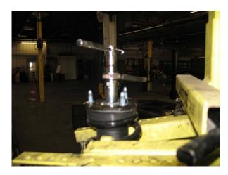
**4c** The new Belltech strut will use the O.E. rubber bump stop. Lubricate the strut shaft and remove the bump stop as shown or by using any similar method. Be careful not to damage the strut shaft during this operation.
