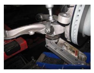
With the use of a floor jack and supporting the lower control arm across its arms, raise the lower control arm back into position, when possible insert a screwdriver or similar device to help align the lower control arm back into the frame points. After this is achieved, you can adjust the floor jack to align each side.
