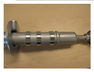
**6a** After selecting the correct number spacers required. Again using a spring compressor. Reassemble all the O.E. components onto the Belltech Lift Strut. The kit includes top stem spacers to be used before the top fastener (nut).
