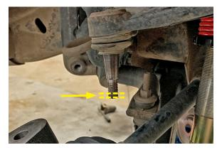
22. 4WD ONLY: Insert drive shaft into hub assembly opening. Ensure splines are properly aligned before continuing.
