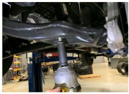
31. Reattach the lower control arm to the frame using the OE alignment hardware. Do not tighten or torque until your vehicle is back on the ground.
