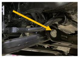
12. Loosen and remove the nuts securing the lower strut mount to the control arm.
