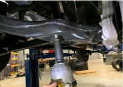
13. Push the spindle and lower control arm down and back until the lower shock studs are clear of the control arm.
