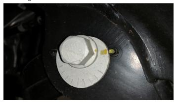
33. Reinstall the sway bar. The bushing bracket will be torqued to 66 lb.ft and the end link nuts will be torqued to 111 lb.ft.
