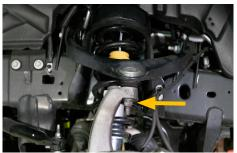
16. Loosen, but do not remove the lower ball joint nut and strike it on the designated areas to separate it from the lower control arm.
