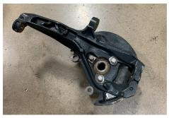
19. Slide the Belltech spindle assembly back onto the lower ball joint. Attach and tighten the lower ball joint nut to OE specifications.
