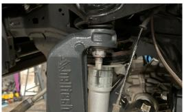
21. Reinstall the ABS line. Route the wire behind the brake backing plate on the spindle.
