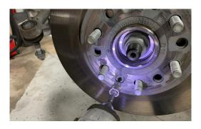
14. Remove the ABS sensor from the spindle using a 5mm hex key.
