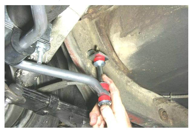
8. Remove the angle bracket from the end link assembly and mount the short leg of it to the frame. Use a half-inch washer between the Nyloc nut and the frame, and another washer between the head of the bolt and the bracket. Re-attach the end link assemblies to the Anti-Sway Bar and the angle brackets as before.
