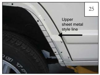
Remove inner pieces. Starting approximately 3" above upper sheet metal style line mark horizontal lines 1.5" apart using a grease pencil or marker.
