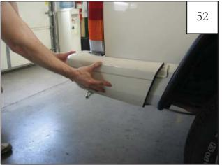
(For 97-01 Model Years Only) If desired, trim bumper piece to fit with flare and reinstall.
