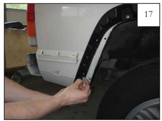
Align outer edge of inner piece P4 (D4 for driver side) with the measuring line made in Step 12. Use a grease pencil or marker to mark the lower rear hole location on the sheet metal.
