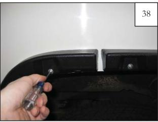
Install flange nuts using a 5/16" socket and wrench and using a #2 Phillips bit for the M5-.8 screws in upper two holes of P3 and upper single hole of P4 (D3 & D4 for driver's side).
