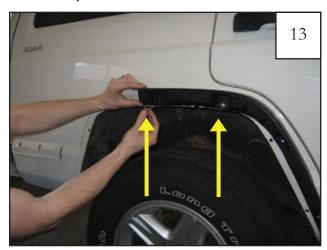
Position inner piece P3 (D3 for driver side) on fender, aligning top two holes in the inner piece with existing factory holes in sheet metal. Slide washer onto M5-.8 machine screw. Insert a screw/washer assembly through inner flare piece and fender and secure with a flange nut. *Only hand tighten at this time.*
