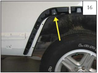
Position inner piece P4 (D4 for driver side) on fender, aligning top hole in the inner piece with existing factory hole in sheet metal. Slide washer onto M5-.8 machine screw. Insert a screw/washer assembly through inner flare piece and fender and secure with a flange nut. *Only hand tighten at this time.*
