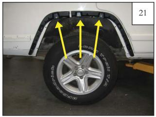
Reinstall inner pieces P3 & P4 (D3 & D4 for driver side) by aligning the parts with the upper factory holes and newly drilled holes. Attach inner piece to the sheet metal with a screw/washer and flange nut in upper hole locations. (3 locations) *Only hand tighten at this time.*
