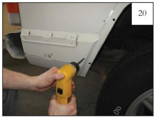
Using a 1/4" drill bit, drill through sheet metal on lower two locations marked in steps 14 & 17. Predrill with a smaller drill bit if desired.
