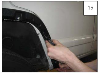
Align outer edge of inner piece P3 (D3 for driver side) with the measuring lines made in Step 10/11. Use a scratch awl to mark the upper front hole location on the sheet metal making sure awl is perpendicular to sheet metal and inner piece.
