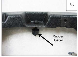
Install screw, washer, spacer combo through inner pieces P3 & P4 (D3 & D4 for driver's side) corresponding with 7/64" holes drilled in step 19. Rubber spacer should be on sheet metal side of inner piece.
