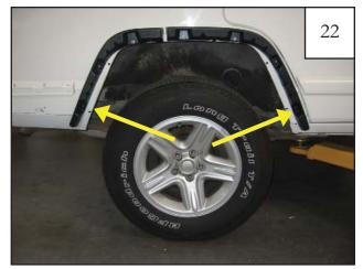
Position inner pieces using supplied tuflocks on lower two hole locations drilled in the sheet metal with the 1/4" drill bit. Do not fully fasten as inner pieces will be removed after marking for trimming.
