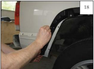
Align outer edge of inner piece P4 (D4 for driver side) with the measuring line made in Step 12. Use a scratch awl to mark the upper rear hole location on the sheet metal making sure awl is perpendicular to sheet metal and inner piece.
