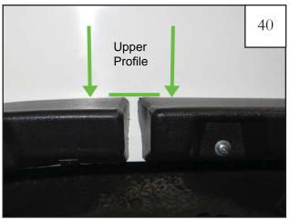
Make sure upper profile of inner pieces match. If not, loosen and realign.
