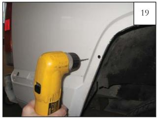
Remove inner pieces from rear fender. Using a 7/64" drill bit, drill through sheet metal on upper two locations marked with a scratch awl in steps 15 & 18.
