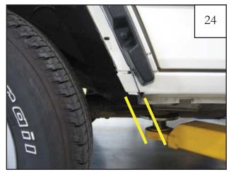
At end of inner pieces extend trimming line so that it is parallel with the wheel well opening instead of following inner piece curvature.
