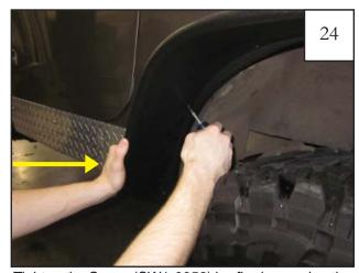
Tighten the Screw (SW1-0056) by *firmly* pressing the flare toward the vehicle while tightening the Screws.
