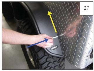
Starting at one end, use the flat edge of the supplied Edge Trim Tool (ET1-0002) to further adhere the edge trim to the vehicle surface. Slide the tool along the edge trim while pressing it in toward the vehicle surface.
