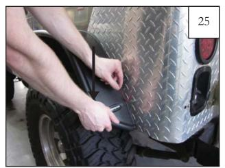
Peel outer tape liner from the Edge Trim (GP1-0006). Push down *lightly* on the fender flare to create a small gap between the sheet metal and the edge trim. This makes it easier to pull the red liner.
