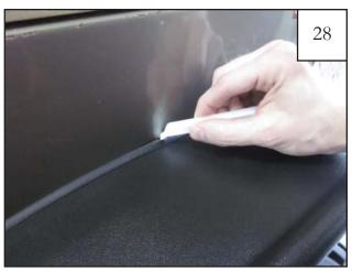
Use the hooked end of the Edge Trim Tool (ET1-0002) to check for full adhesion. Do this by sliding it along the top of the edge trim to visually verify that the tape is adhered to the vehicle surface. Repeat Step 27 if the tape is not fully adhered to the vehicle surface.
