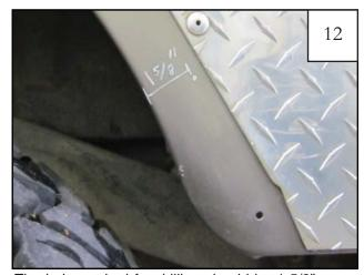
The hole marked for drilling should be 1-5/8" away from (and perpendicular to) the wheel well opening. Adjust mark for drilling as needed.
