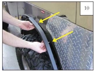
To attach inner piece D4 (P4 for passenger side) you will need to drill 1 new hole location in the sheet metal. Do this by first placing inner piece D4 on vehicle using only top 2 screws in order to align for marking of lower fastening hole.
