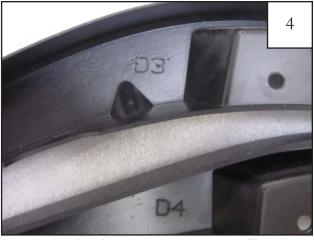
Locate the flat flare rear inner pieces. The driver side rear inner pieces are marked D3 & D4. The passenger side rear inner pieces are marked P3 & P4.
