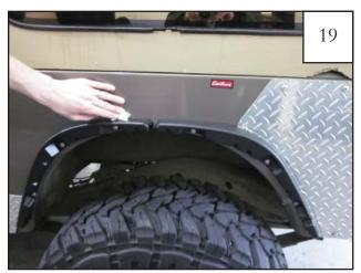
Use one supplied Wipe (AD1-0008) to clean the *sheet metal* above each inner piece in preparation to tape the edge trim to the sheet metal. *This must be done for proper flare installation.*
