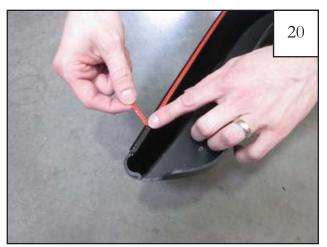
Peel back 1-2" of red liner on each end of the Edge Trim (GP1-0006) and bend toward the outside of the flare.
