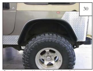
Completed rear driver's side flare installation.
