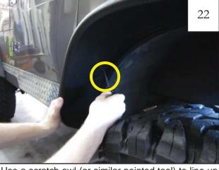
Use a scratch awl (or similar pointed tool) to line up the Clips (CL1-0022) with the outer flare holes (6 locations). If needed, use a flashlight to better locate the Clips.
