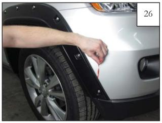
Remove the red tape liner from edge trim. *Note: Be careful not to tear red tape liner during the removal processs.*
