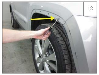
Use a pry tool to remove any remaining factory fasteners that may have stayed on the vehicle during the removal process. Straighten the front wheels once all fasteners have been removed.
