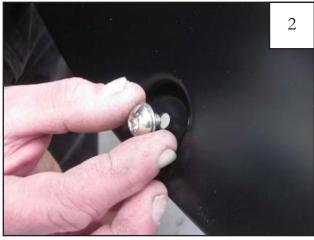
Put each Bolt/Washer combination through a pocket hole in the flare, with the Bolt head and Washer on the outside.
