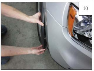
Starting at the front end of the factory flare, firmly grip part and pull to remove from vehicle. *Note: You will hear popping sounds as the factory fasteners release from vehicle. This is normal.*
