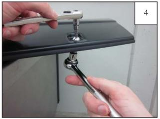
Fully tighten using an 8mm wrench or 3/8" ratchet with an 8mm socket for the Nyloc Nut and use the supplied Torx Bit (SW1-0052) and wrench for the Bolt. Repeat for remaining pockets.
