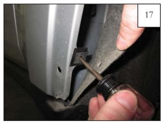
Using an awl tool, make a hole thru each Black Tab using the hole in the clip as a guide. Replace factory wheel well liner to original position.
