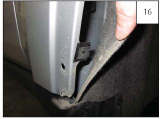
Place supplied Metal Clip (CL1-0022) over Black Tabs installed in step 15. The hole in the Clip should align with the factory hole in the sheet metal covered by the Plastic Black Tab.
