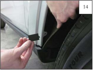
Pull back wheel well liner to expose factory holes in sheet metal. A supplied Plastic Black Tab (MT1-0014) will be installed over the factory holes. See next step.
