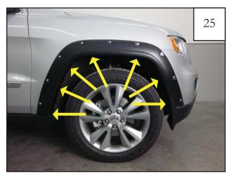
Screw/Clip locations (7 places). Ensure flare is properly aligned on vehicle and fully tighten all fasteners using a #2 Phillips Stubby Screwdriver
