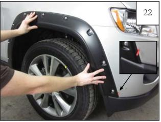
Hold the front Flare onto vehicle ensuring tape liners are exposed.
