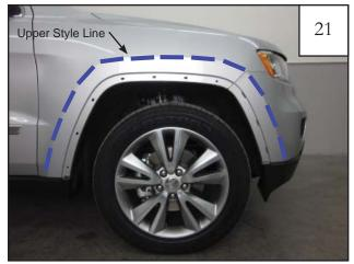
Using provided Alcohol Prep Pad (AD1-0010), clean sheet metal of fender and bumper for front flare installation. Use upper style line on fender as a guide.
