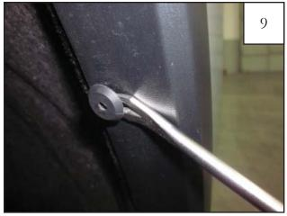
Using pry tool, remove factory fasteners drilled in previous step.
