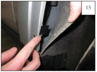
Pull adhesive liner from supplied Plastic Black Tabs (MT1-0014) and fold over the factory hole locations to cover and adhere to each side of the sheet metal (5 places refer to Step 13).
