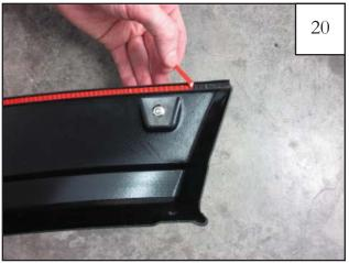
Pull back 1-2 inches of tape liner from each end of installed edge trim and fold towards outside of the flare.
