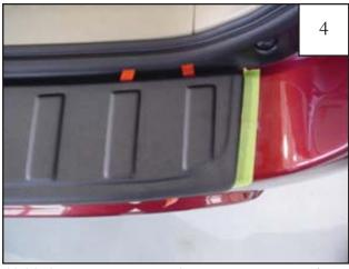
Hold the part at an angle to prevent tape from prematurely sticking, and align the part on the bumper by centering bump in rear door sill between two center ribs in part and using the masking tape applied in Step 1 as a guide.
