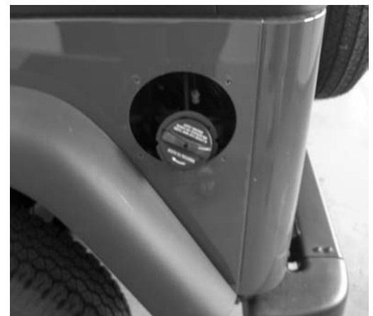
Figure #1 – Remove Gas Tank Outer Flange
