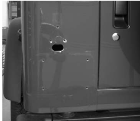
Figure #2 – Remove Tail Light & License Plate
