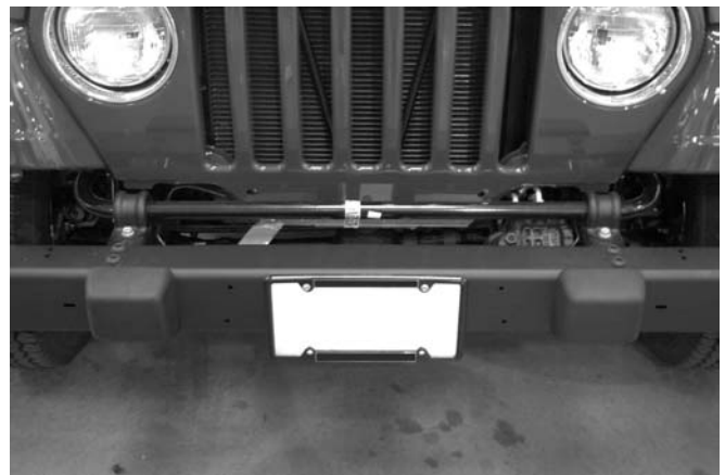
Figure #8 – Factory Front Panel Removed
