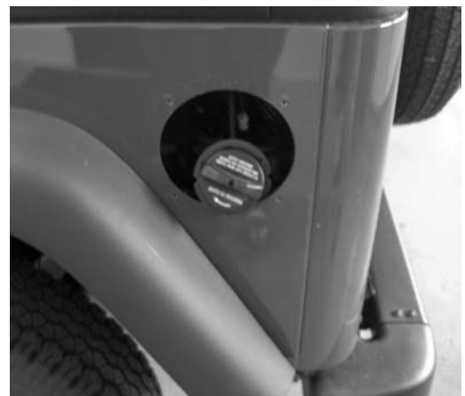
Figure #1 – Remove Gas Tank Outer Flange
