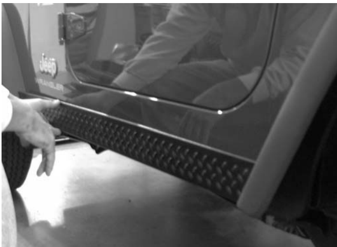
Figure #7 – Install Side Panel
