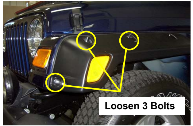
Photo #2 – Loosen Bolts (Do NOT Remove)
