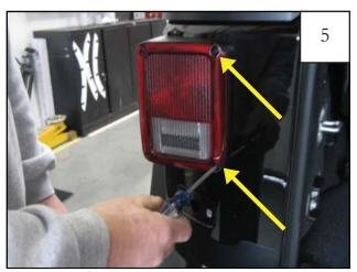
Using a #2 Phillips screwdriver, remove two screws closest to the inside of the vehicle.
