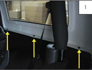
Using a T-40 Torx bit and a 3/8" ratchet remove six bolts fastening hard top to vehicle (3 bolts per side) and save bolts for reinstallation. With a partner, remove hard top from vehicle.
