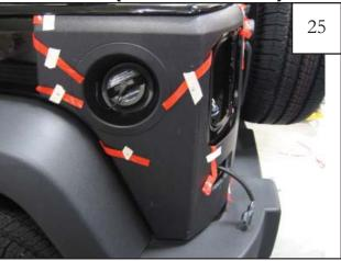
Position the part on the vehicle so it fits around the gas door. Then, using a #2 Phillips screw driver, reattach the tail light.
