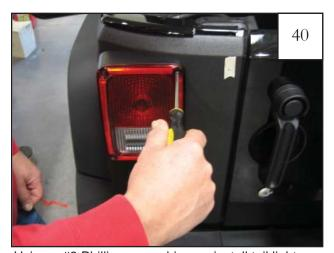
Using a #2 Phillips screwdriver, reinstall tail light.
