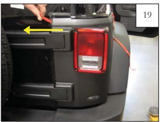
Pull tape liner 7 to the left toward the driver side of the vehicle. *NOTE: Refer to steps 8 & 9 for tape liner tab numbering.*
