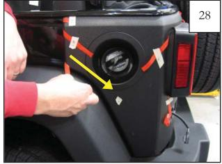
Pull tape liner 3 downward on a slight diagonal matching the curvature of the part. NOTE: Refer to step 24 for tape liner tab numbering.
