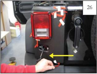
Pull tape liner 1 to the left toward the driver side of the vehicle. *NOTE: Refer to step 24 for tape liner tab numbering.*
