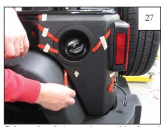
Pull tape liner 2 downward on a slight diagonal matching the curvature of the part. NOTE: Refer to step 24 for tape liner tab numbering.
