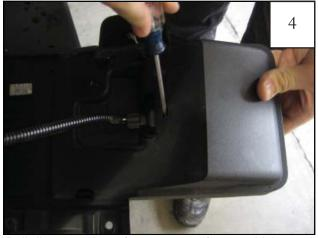
Pull license plate frame away from vehicle and disconnect the frame by using a small screw driver or similar tool inserted in the hole and pressing down on the connector to pop it out.
