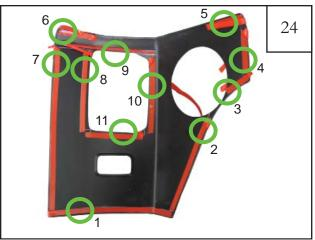
Using a marker, label the tape tabs with the numbers 1-11 as shown. Using masking tape, tape each tab on the outside of the part.
