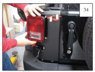
Using a #2 Phillips screwdriver, remove the tail light.
