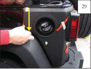
Pull tape liner 4 downward. NOTE: Refer to step 24 for tape liner tab numbering.
