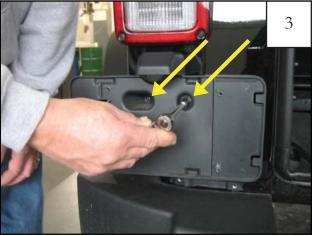
Using a 7mm socket with a 1/4" ratchet and 1/4" extension, remove two bolts from the face side of the license plate frame.
