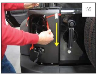
Pull tape liner 8 downward. NOTE: Refer to step 24 for tape liner tab numbering.
