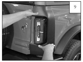
Apply FIRM pressure to all flanges to ensure proper adhesion.
