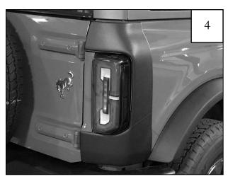
Test fit the Corner Guard in place. Take note of where the red tape liner aligns with the vehicle body.
