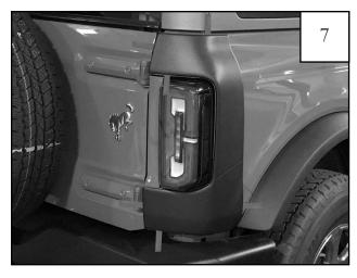
Position the Corner Guard in place and align with the previously cleaned surface. Ensure that the red tape pull tabs are all accessible. Apply pressure to exposed tape.
