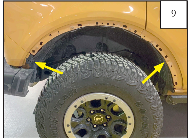
Remove (2) fender liner fasteners and retain.
