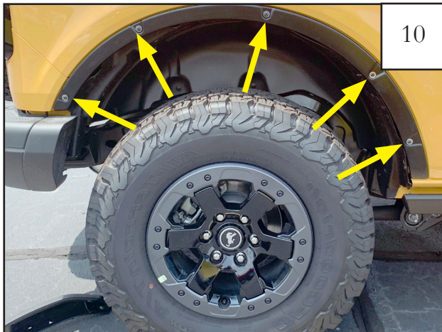
Install fender delete using (5) 133606M bolts, (10) WA1-0029 washers, and (5) NU1-0015 nuts. (See diagram Step 11)
