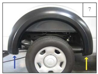
Using a 10mm socket wrench, tighten 35mm bolt through spacer and factory hole in sheet metal.
