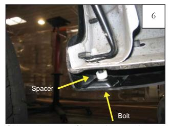
Slide supplied spacer (SP1-0003) between flare and sheet metal. Thread supplied 35mm screw (SW1-0025) through hole in flare, through spacer, and through factory hole in sheet metal. See Step 7.
