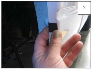
Wrap a black tab (MT1-0014) around the wheel well sheet metal, centered over each of the four marks made in Step 2.
