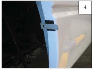
Install supplied clips (CL1-0009) over each of the four black tabs placed on the sheet metal in Step 3.
