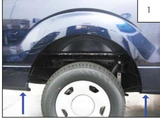
Remove two factory bolts with a 10mm socket wrench and disgard. (Note: New hardware is supplied, see Step 6)
