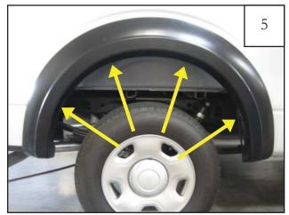
Hold flare to vehicle and start supplied truss head screws (SW1-0058) through the two topmost holes in wheel well. Then start supplied truss head screws (SW1-0058) through remaining two holes in flare. Tighten all screws.
