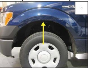
Install Clip (CL1-0011) over fender wheel well lip. See Step 6.
