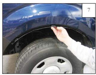
Line up the holes in the inner piece with the two uppermost factory holes and the Clip (CL1-0011). NOTE: Driver's side inner piece is marked with an "L" and passenger's side inner piece is marked with an "R".
