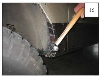
Push splash shield back into wheel well then, using a hammer, bend the tabs of sheet metal into fender well as shown. Replace upper factory bolt removed in Step 4.
