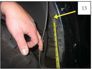
At Pinch weld (inside splash shield), measure up 9" and make a mark. *NOTE: the pinch weld will not be cut, it will be hammered flat.*
