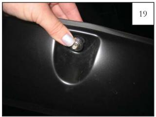
Insert a kit-supplied Screw (SW1-0045) through a pocket hole on flare.
