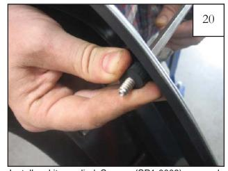
Install a kit-supplied Spacer (SP1-0009) on each Screw from the backside of the pocket using drill with supplied Torx Bit (SW1-0052). Screw threads must protrude through spacer for proper attachment of flare. Repeat for all pockets.
