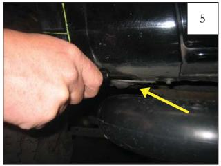
Use a trim tool to remove one plastic fastener located at bottom rear of splash shield (next to bottom of door seam).
