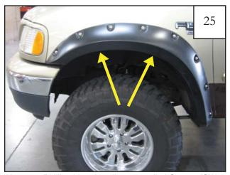
Use a #2 Phillips bit to install two supplied Screws (SW1-0066) through fender flare and into sheet metal of wheel well at locations shown (there are pockets in fender flare at these locations)
