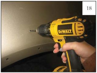
Remove flare and drill hole locations with a 3/16" drill bit, making sure to keep the drill level and perpendicular to fender surface.
