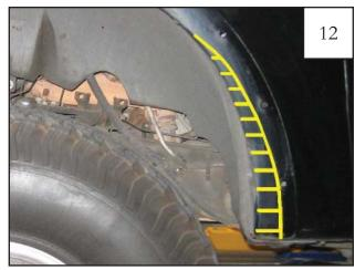
At 1-1/2" intervals, make horizontal lines from fender lip to line drawn in Step 11. These lines will be cut later, forming tabs to be hammered in.
