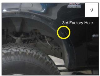
Third factory hole location. If the truck did not come with factory flares and there are no factory holes on fender, refer to Step 10.
