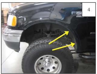
Use a 7/32" socket to remove two bolts fastening the splash shield to the fender well. Retain one bolt for reinstallation in upper hole after cutting sheet metal.
