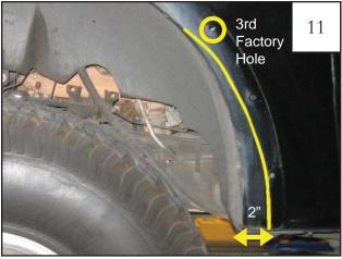
Draw a line from mark made in Step 7 up to mark made in Step 8 or Step 10, curving gradually to connect the marks. The line should be as shown.
