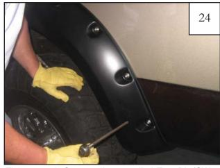
Tighten each Screw using supplied Torx Bit (SW1-0052) at 24 in·lb (2 ft·lb) speed. *Over-tightening screws may cause them to strip!*
