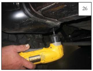
Install one supplied Screw (SW1-0056) through the lower rear pocket in fender flare and into sheet metal.
