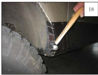
Using a hammer, bend the tabs of sheet metal into fender well as shown.
