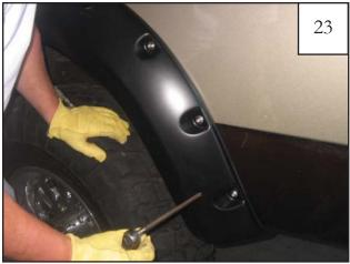
Holding the flare in position on fender, align and start the Screws through the holes in the vehicle. *Make sure edge trim isn't folded over before tightening screws.*
