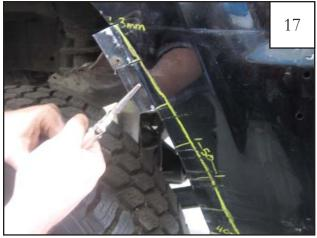
Cut horizontal lines made in Step 9 & Step 14. Use pliers or vise grips to bend the sheet metal tabs straight.
