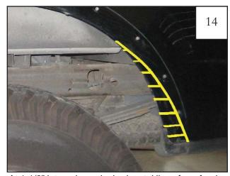
At 1-1/2" intervals, make horizontal lines from fender lip to line drawn in Step 13. These lines will be cut later, forming tabs to be hammered in.
