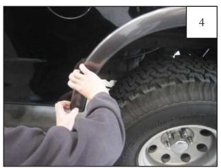
Starting at front of flare, pull firmly to release flare from fender, working your way to the back. You will hear popping noises as clips release. It is O.K. if clips break, they will be discarded.
