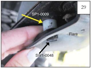
At lower REAR underside of flare, slip a supplied Spacer (SP1-0009) between flare and bumper (spacer is white in picture for visibility). Then install a supplied Bolt (SW1-0048) through hole in flare and spacer, and into bumper skin.
