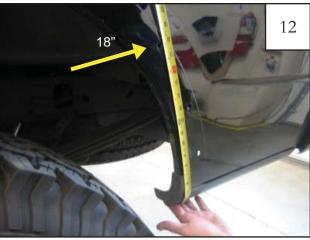
For trucks without factory flares ONLY: Wrapping tape measure up from underside of fender, measure up 18" and make a mark on fender lip where tape measure intersects.
