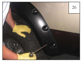
Tighten each Screw using supplied Torx Bit (SW1-0052) at 24 in·lb (2 ft·lb) speed. *Over-tightening* screws may cause them to strip!
