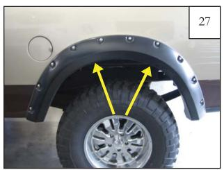
Use a #2 Phillips bit to install two supplied Screws (SW1-0066) through fender flare and into sheet metal of wheel well at locations shown (there are pockets in fender flare at these locations)
