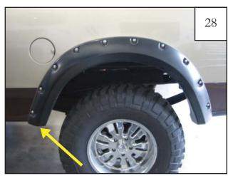
Install one supplied Screw (SW1-0056) through the lower FRONT pocket in fender flare and into sheet metal.
