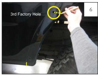
At fender lip, make a mark horizontal to the third factory hole up from bottom front of fender well.
