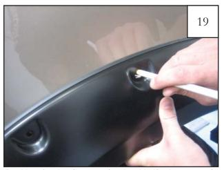
Position fender flare on fender. Verify that parts fit and no additional cutting is needed. Maintaining part position, mark the hole locations in the fender using the holes in the flare as guide (10 places).
