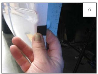
Wrap a Tab (MT1-0014) around the wheel well sheet metal, centered over each of the four marks made in Step 5.
