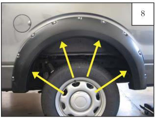
Hold flare to vehicle and start Screw (SW1-0058) through the two topmost holes in wheel well. Then start Screws through remaining holes in flare. Tighten all Screws.
