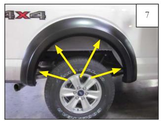
While holding flare to vehicle, start supplied screws (SW1-0058) through the four topmost mounting holes in flare and into the clips installed in Step 5.
