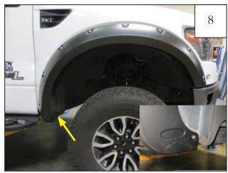
Re-install factory screw in hole at the bottom rear of the flare and into the factory hole.
