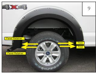
Reinstall two factory 7mm screws. Install two Panel Retainers (RV1-P008).
