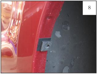
Install a Clip (CL1-0005) over each of the three Tabs (MT1-0014) placed over the upper 3 marks made in Step 6.
