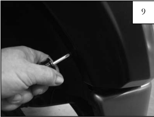
Still holding flare to fender, install supplied black plastic retainers (RV1-P001) using a Phillips screw driver. See step 10.
