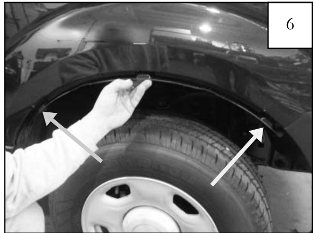
Using a 7/32" socket wrench, reinstall the factory screws through the inner piece.
