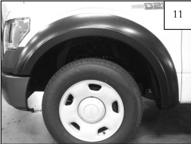
Completed front flare installation.
