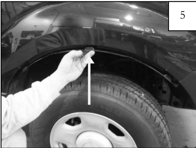
Using a Phillips screw driver, start a pan head screw (SW1-0056) through center hole in inner piece and through the speed clip over the fender wheel well lip.
