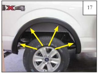
While holding flare to vehicle, start supplied screws (SW1-0058) through the four topmost mounting holes in flare and into the clips installed in Step 15.
