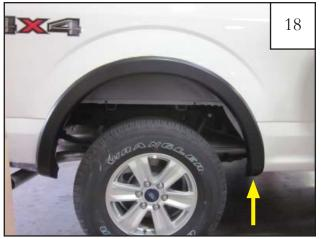
Start a supplied screw (SW1-0050) through the flare into the clip installed in Step16. Tighten all screws.
