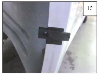
Install a Clip (CL1-0009) over each of the four Tabs (MT1-0034) placed over the upper 4 marks made in Step 13.
