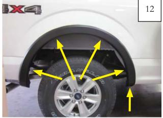
Hold flare to vehicle and mark five flare hole locations with a grease pencil.
