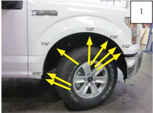
Remove five factory screws with a 7/32" socket wrench. Remove two rear most factory screws with 9/32" socket wrench. *Save screws for reinstallation*.
