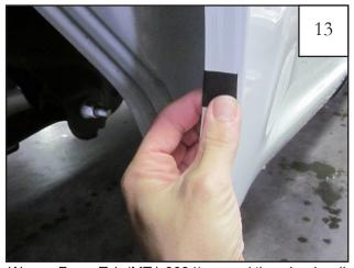
Wrap a Foam Tab (MT1-0034) around the wheel well sheet metal, centered over each of the upper four marks made in Step 15. Place a Mylar Tab (MT1-0014) at the mark made on the lower front of the wheel well (see step 14).
