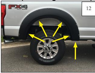
Hold flare to vehicle and mark five flare hole locations with a grease pencil.
