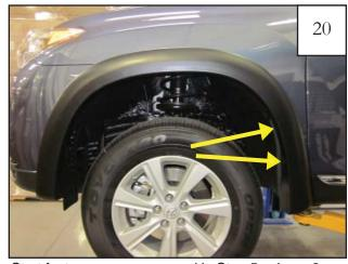
Start factory screws removed in Step 5 using a 3mm Allen Wrench. *Do not tighten*.
