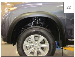
Install a Tuflock (RV1-P001) through flare and into sheet metal of wheel well where rear and lowermost plastic factory fastener was removed in Step 7.
