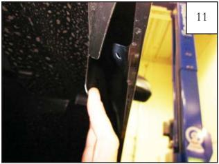
Install Tab (MT1-0017) over factory hole locations behind wheel well liner. *Reference Step 8 for locations*.
