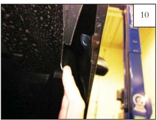
Pull wheel well liner out from behind fender lip.
