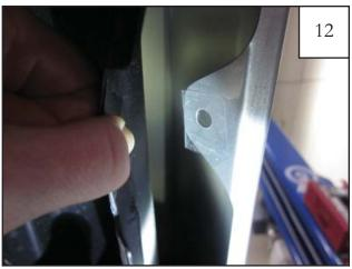
Slide Clip (CL1-0022) over factory hole locations behind wheel well liner over tab installed in previous step. Two locations. *Reference Step 8 for locations*.
