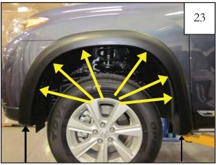
Once all hardware is started, check flare for proper positioning. Apply pressure at each fastening point and tighten all screws and bolts.
