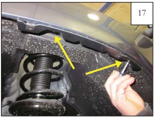
Hold front flare inner piece in wheel well with angled hole locations aligned with clips installed in Step 12. Using a #2 Phillips Screwdriver, install Screws (SW1-0058) through front flare inner piece, through wheel well liner, and into Clip. Make sure that the corners of the Front Inner Piece are mounted flush with the sheet metal.
