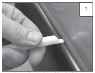
Using flat end of supplied Edge Trim Tool (ET1-0001), seat edge trim against flare by inserting straight end between edge trim and flare at one end. Next, slide around entire edge to the other end.
