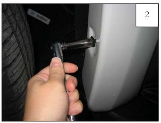
Start a supplied Hex Screw through top rear hole in flare and into factory hole in rear of wheel well.
