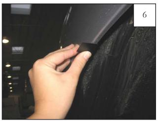
Remove flare from fender. Center a supplied Black Tab over each mark made in Step 4.
