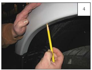
Hold the front of the flare firmly on the fender. Starting with the second hole from the front of the flare, mark three clip locations with a grease pencil.
