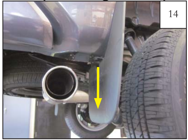
Remove push retainer from underside of factory mud guard and remove mud flap.
