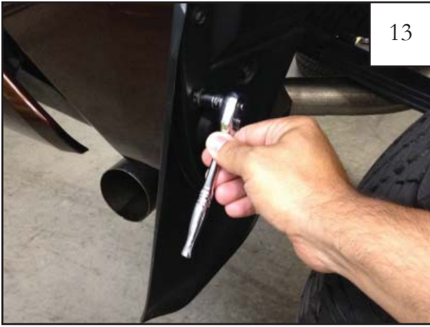
Using a socket wrench with a 10mm socket, factory screw second from the top of the mud guard.
