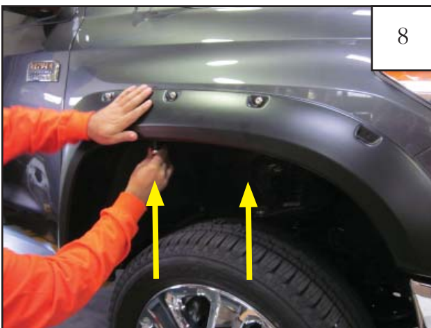
Place flare on fender, aligning holes with clips on the bracket. Start two supplied 20mm Hex Screws (SW1-0036) through two holes on the top of the flare and into clips.
