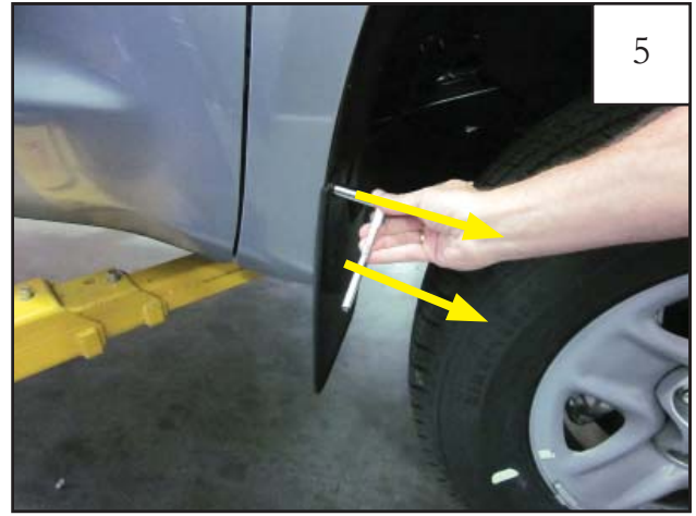
Using a 10mm socket, remove two factory screws from factory mud guard as shown.
