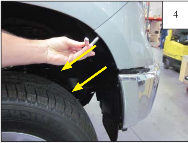
Using a 10mm socket, remove two factory fasteners from front of wheel well.
