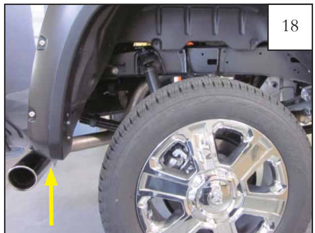
Install supplied Push Retainer (RV1-P009) into factory hole on underside of flare.
