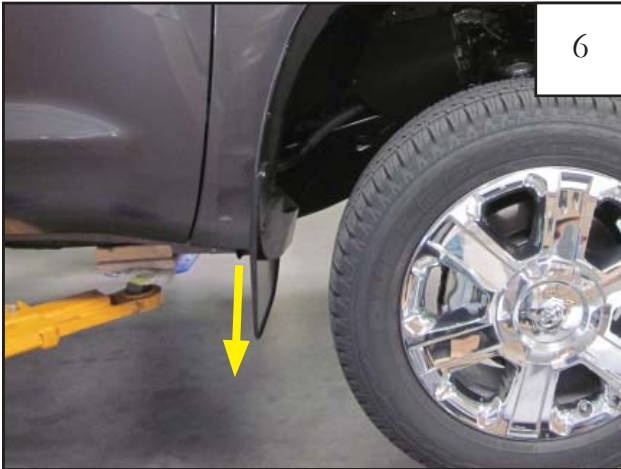
Remove push retainer from underside of factory mud guard. Remove Mud Guard from Vehicle.
