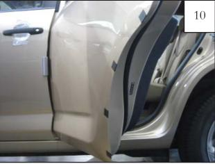
Remove door piece from door. Center a supplied black tab over each mark made in step 8.
