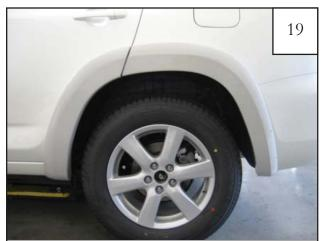
Close vehicle door and check alignment of door piece to rear main flare.
