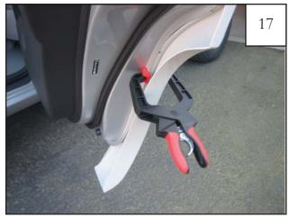
Once center two screws are installed, tighten the uppermost and lowermost screws. *Note: The pressure applied by the clamp or partner may have to be moved from the center so that the plastic is fully set in the clip for the uppermost and lowermost clip locations.*
