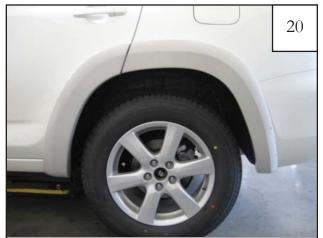
Adjust rear main flare for proper alignment. Once satisfied, tighten all rear main flare screws using a right angle #2 Phillips stubby screwdriver
