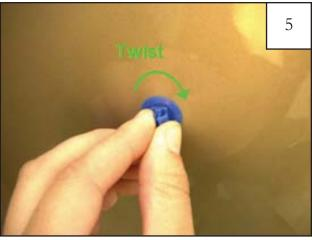
Using a clockwise twisting motion, remove eleven factory plastic clips from fender. See Step 7.
