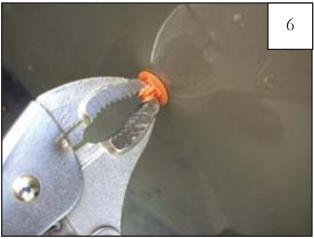
Remove one clip from fender using vise grips, pulling with a rocking motion. See Step 7.
