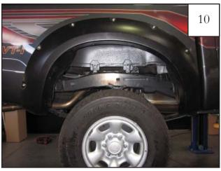
Position flare on fender and re-install factory screws through holes in flare and into factory holes.
