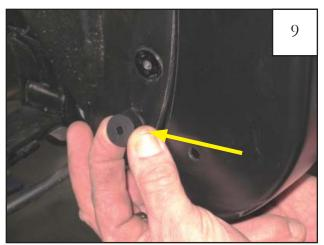
Install supplied grommet (GR1-0001) into factory hole.
