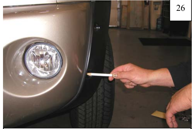
Using a grease pencil, mark hole locations for Front Bumper Piece pockets (2 places).
