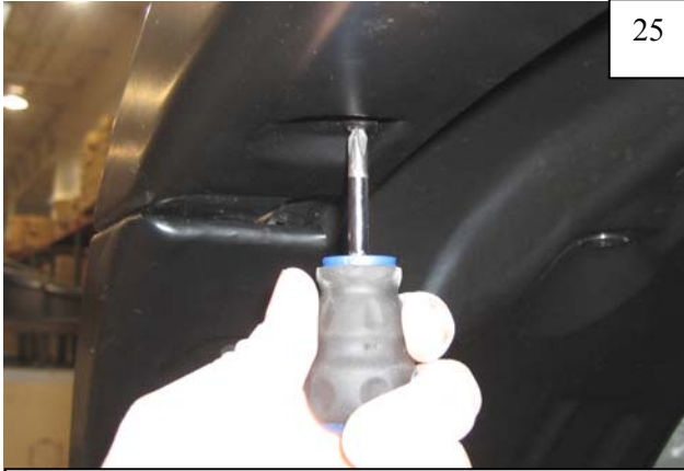
Install a supplied Serrated Flange Screw through hole in flare and into clip installed in Step 23 (4 places).
