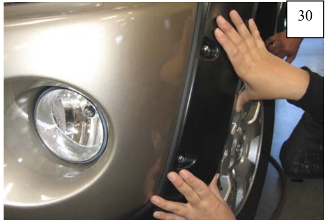
Situate flare on bumper, inserting screws through holes drilled in bumper in Step 27.
