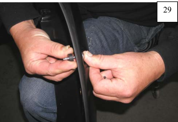
Install Screw/Washer Assembly through pocket holes drilled in Step 12. Place a supplied black spacer on the back of the screw.
