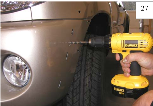
Remove fasteners installed in Steps 24 – 25 and remove flare from fender. Drill at marked places with a 5/16" bit.
