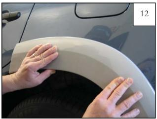
Replace flare on fender, aligning holes with holes in clins
