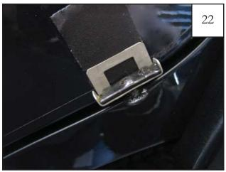
Hand start serrated-flange screws through each clip. The end of the shaft should be flush with the uppermost edge of the clip.
