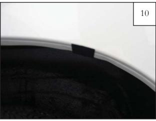
Remove flare from fender. Center a supplied black tab over each mark made in step 9.
