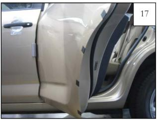
Remove door piece from door. Center a supplied black tab over each mark made in step 16.
