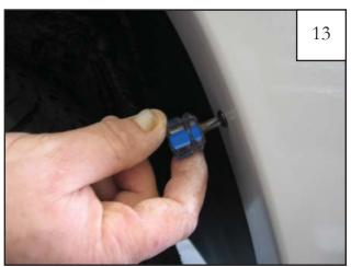
Start supplied serrated-flange screws through holes in flare and into the "S" clips installed in step 11. *Note:* Do not tighten screws until door piece is installed.
