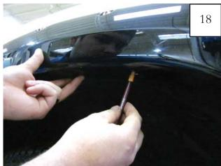
Hold the flare firmly on the fender. Using a grease pencil, mark two clip locations using existing holes in flare. See step 19
