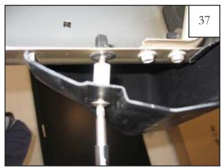
At bottom rear of flare, install a supplied Screw (SW1-0034) and a Spacer (SP1-0008).
