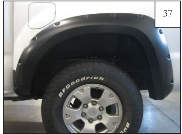
Completed rear flare installation.
