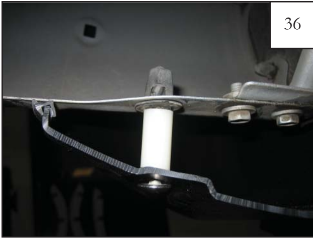
At bottom rear of flare, fasten flare to vehicle with a supplied 1-3/4" #14 Truss Head Screw (SW1-0034) through a 1" Spacer (SP1-0005).
