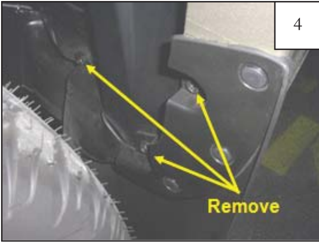
Remove three factory screws from the mud flap. Save screws for reinstallation.
